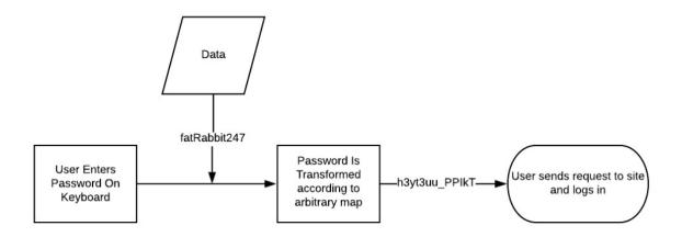
The above illustrates how a user would physically press keys that are in their usual layout on their keyboard, once the keys are entered, each character is simply substituted for an alternative, according to a unique randomly generated character mapping scheme. This is a substitution cipher. The diagram below illustrates a simple substitution cipher.
