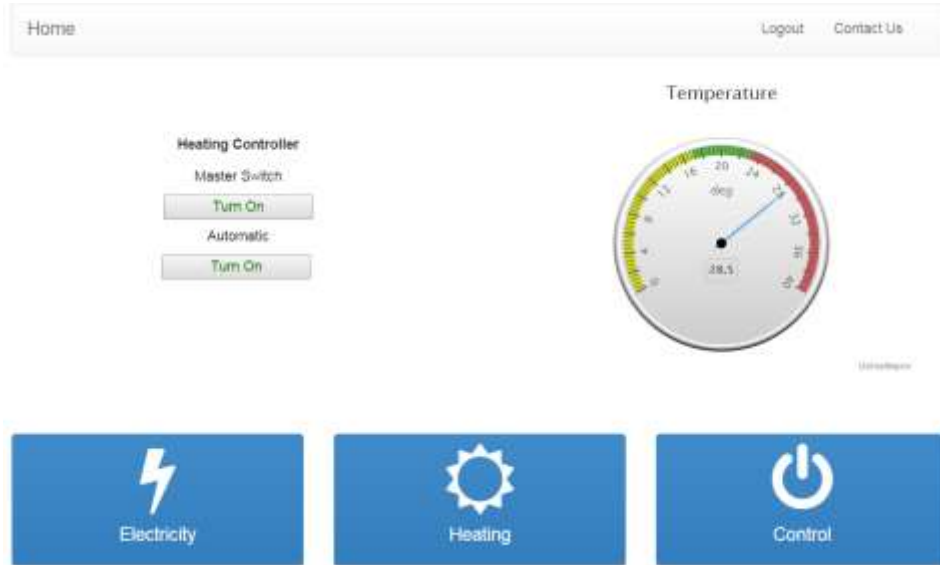
Fig. 6 Heating Screen - Off Mode
