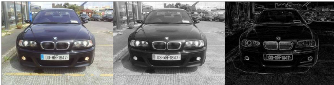
Figure: Three images: Initial image, Gray scale image, Gray scale Image with Edge Detection
