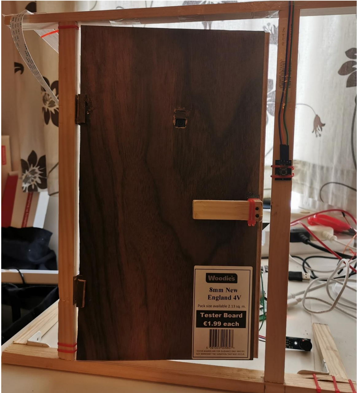
Figure 17 door access hardware implementation front
