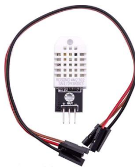
Figure 2 temperature & humidity sensor
